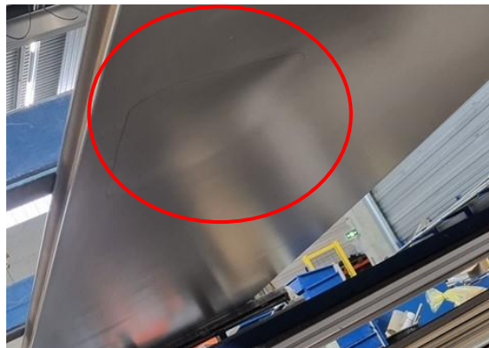
Fig. 2: Extensive delamination and blistering of type 3 components after storage at 80°C for 14 days.
